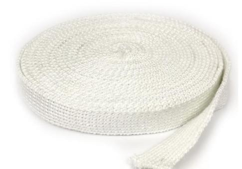
PRODUCT INFO: White high temperature flat tape that can withstand continuous temperatures of 1000F. No self adhesive. Apply with high temperature silicone or stove cement.
