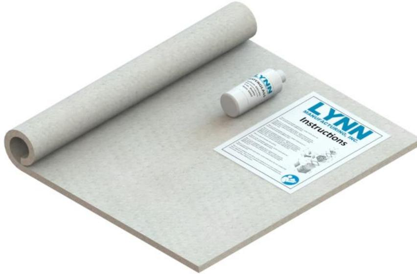
**PRODUCT INFO:** Combustion chamber floor insulation blanket or base liner for oil-fired or gas-fired boilers. Made from 2300F rated ceramic fiber. Comes with instructions how to cut to size for common applications. Also comes with waterglass to adhere
