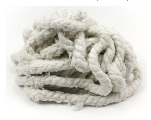
PRODUCT INFO: Ceramic fiber rope that can withstand continuous temperatures of 2300F. Twisted ply type. Cream colored. Made from alumina-silicate based ceramic fiber.
