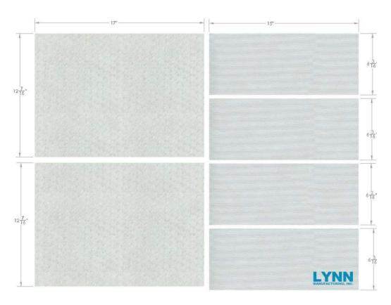
2728C KIT CONTAINS: Exact fit replacement for Ironstrike H8022. Kits contains 4 boards and 2 blankets.
