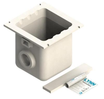
KIT CONTAINS: Combustion chamber 337350, chamber support board, refractory cement, instructions. Combustion chamber is 19 3/8" x 19-3/8" x 18" and 1" thick.
