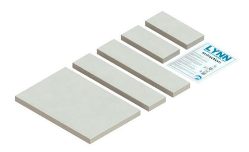
KIT CONTAINS: Replaces 62072006 flue box insulation kit. Contains door insulation 82072008 (16-1/2" x 11-1/8" x 1 molded ceramic fiber board), side insulation 7207202 (9-3/16" x 3-13/16" x 1" molded ceramic fiber board x 2 per kit), top & bottom in
