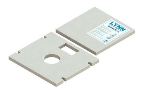
KIT CONTAINS: Replaces 62072001 insulation kit. Contains front insulation 82072013 (17-1/4"  $\times$  15-1/2"  $\times$  1 molded ceramic fiber board), floor insulation 1033204-01 (14-1/8"  $\times$  14-5/8"  $\times$  1" molded ceramic fiber board), instructions
