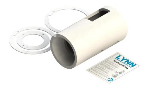
PRODUCT INFO: Combustion chamber replaces Nordyne 903423. Vacuum cast ceramic fiber chamber rated to 2300F. Kit also contains HE Gasket 689528 and burner gasket 660604. Chamber dimensions 7-3/4" OD x 14-13/16" tall x 1/2" thick.
