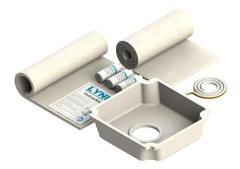
KIT CONTAINS: Replaces Weil-McLain kit 385-700-220 and 591-000-070. Fits all 78 and 80 series boilers with 4" burner. Kit contains: front refractory with 4" opening 591-000-070, rear target wall blanket, floor blanket, rope to seal door, waterglass, i
