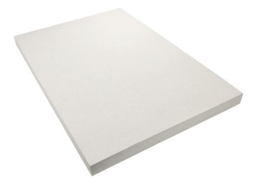
PRODUCT INFO: Vacuum cast ceramic fiber refractory board rated to 2300 degrees Fahrenheit. 16 lbs/ft2 density. Material has low thermal conductivity, low thermal mass and resists thermal shock.
