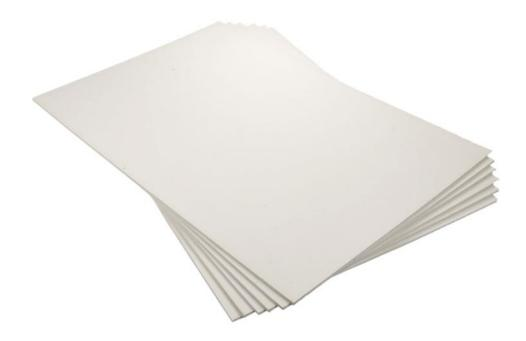
PRODUCT INFO: Vacuum cast ceramic fiber refractory board rated to 2300 degrees Fahrenheit. 16 lbs/ft3 density. Material has low thermal conductivity, low thermal mass and resists thermal shock.
