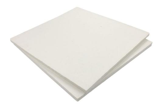
PRODUCT INFO: Vacuum cast ceramic fiber refractory board rated to 2300 degrees Fahrenheit. 16 lbs/ft3 density. Material has low thermal conductivity, low thermal mass and resists thermal shock.
