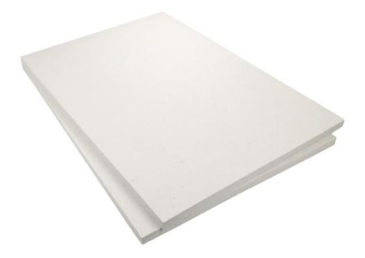
PRODUCT INFO: Vacuum cast ceramic fiber refractory board rated to 2300 degrees Fahrenheit. 16 lbs/ft3 density. Material has low thermal conductivity, low thermal mass and resists thermal shock.
