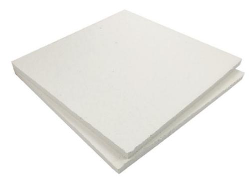
PRODUCT INFO: Vacuum cast ceramic fiber refractory board rated to 2300 degrees Fahrenheit. 16 lbs/ft3 density. Material has low thermal conductivity, low thermal mass and resists thermal shock.
